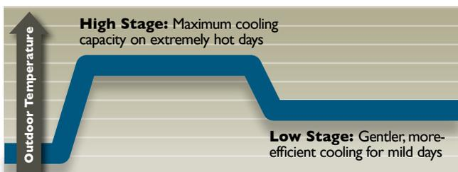
With its two-stage design, the 4SHP16LS makes the distinction between mild and extremely hot or cold days, using only the energy necessary to keep you comfortable.
